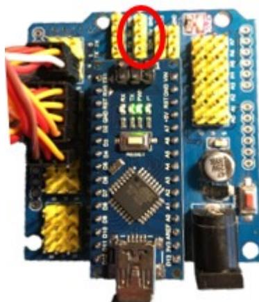
Connect the plug from the tilt sensor so that the black wire is located next to the GND pin. The white wire should be next to the pin marked SDL as shown.
